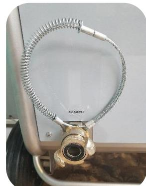
\* is standard medium air with a minimum air supply pressure of 5 bar, required for the correct functioning of the pneumatic parts.
